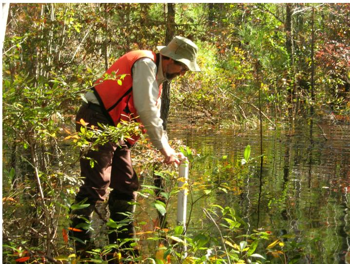
CISA PI Dan Tufford checking a monitoring well at a geographically isolated wetland in Marion County, SC. This work was part of an EPA-funded project to better understand the occurrence and ecological functions of this type of wetland.
